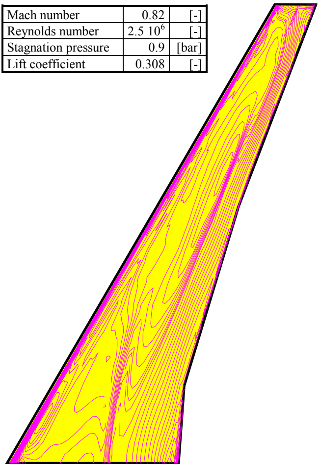
Fig. 8: Contour plot for isobars (upper side); result from fluid/structure coupling.
