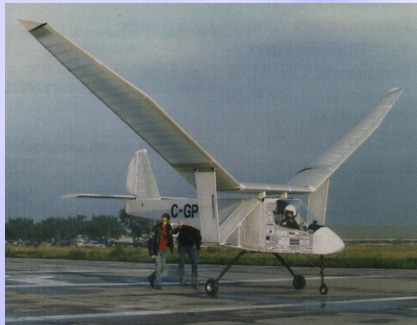
Full-Scale Piloted Ornithopter Prof. J.D. DeLaurier - University of Toronto
